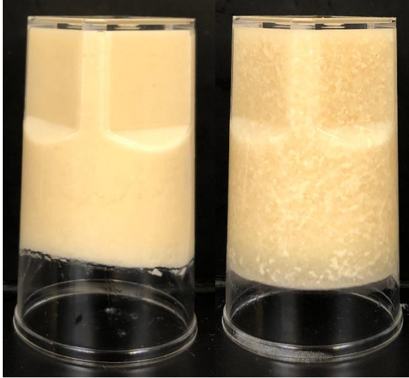
Figure 3.1. Appearance of SL:SA+WPC (left) and SA+WPC (right) bigels.
